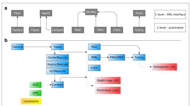
Fig. 1 The simplified architecture of the core MicMac modules. a the low-level and high-level modules dependencies, b the processing workflow. Marked in red are the outcome products, in green are the direct georeferencing inputs
