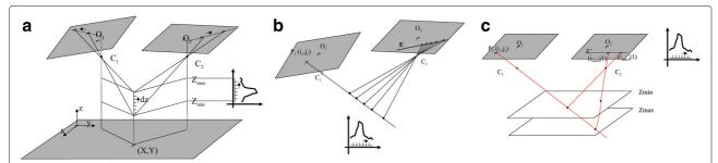
Fig. 3 Three restitution geometries in MicMac. a ground, euclidean space, **b** image geometry discretised along the ray, no resampling **c** image space resampled to epipolar geometry. For a range of the potential Z-coordinates/depths/disparities the similarity measure is computed and further passed to the energy minimization solver
