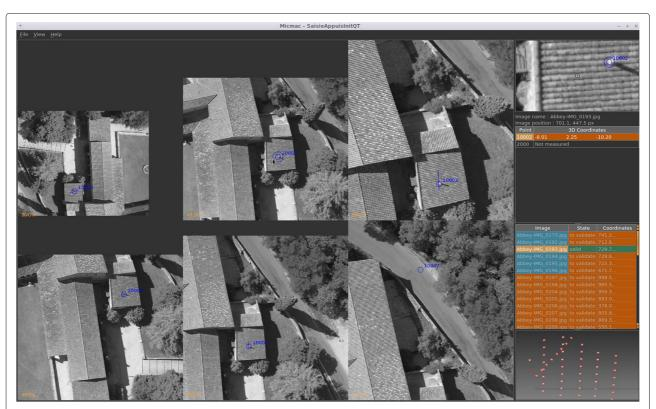
Fig. 11 Interface for measuring GCPs in images
