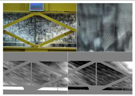
**Fig. 5** Under induced force the concrete beam deformed, while a still camera measured the displacements in during the breaking phase. *Upper left*: the full view image, *upper right*: a close-up of the concrete structure, *bottom left*: displacement in the x-coordinate (max amplitude  $\frac{1}{4}$  pixel), *bottom right*: displacement in the y-coordinate (max amplitude  $\frac{1}{4}$  pixel)
