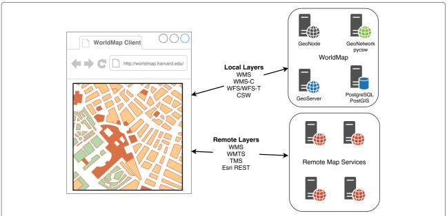
**Fig. 1** Local and remote layers in WorldMap. Local layers are stored in GeoNode and loaded in the client using OGC standards implemented by GeoServer. Remote layers are exposed by a number of web map services using OGC standards or open protocols
