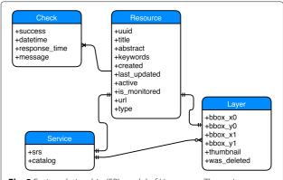
**Fig. 2** Entity-relationship (ER) model of Hypermap. The main Hypermap entities are services, layers and checks. There is a 1-n cardinality between services and layers, service and checks and layers and checks
