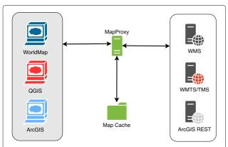
**Fig. 6** Architecture of Hypermap map cache component. The map cache component, MapProxy, acts as a proxy to the external map services and provides a quick access tiles cache with support to the spatial reference systems used in the WorldMap client
