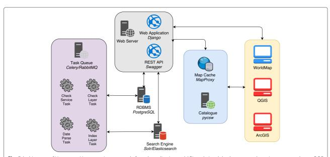
**Fig. 5** Architecture of Hypermap. Hypermap is composed of a web application and API, a relational database, a search engine, a map cache, an OGC catalogue and a task queue. The mapping clients interact with the Hypermap components using standards over http requests
