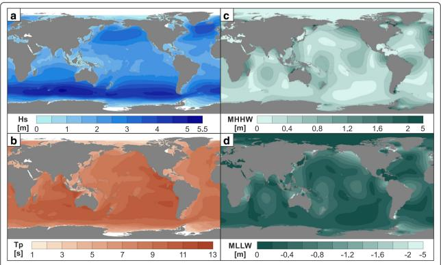
Fig. 2 Global grids of the wave conditions and tidal datums. a Mean significant wave height (Hs); b Mean wave period (Tp); c Mean Higher High Water (MHHW); d Mean Lower Low Water (MLLW)
