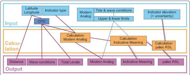
**Fig. 3** Flow diagram showing the relations between the input and output values. Red lines represent the calculation using the Coastal Point Database (CPD, see text for details), blue dotted lines the calculation with an own modern analog
